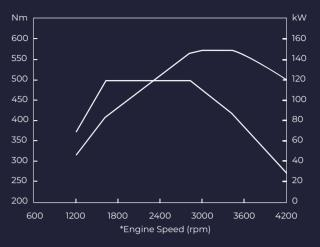
THE NEW GENERATION 2.8-LITRE DIESEL ENGINE (LGD-FTV) HAS BEEN FINE-TUNED FOR INCREASED POWER AND FUEL EFFICIENCY. THE VARIABLE NOZZLE TURBOCHARGER AND THE INTERCOOLER HAVE BEEN IMPROVED, RESULTING IN INCREASED POWER AND TORQUE PRODUCTION, AS WELL AS IMPROVED FUEL ECONOMY.
