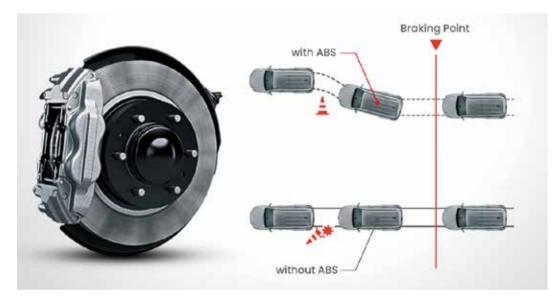
ANTI-LOCK BRAKING SYSTEM (ABS), WHEREBY EXCESS BRAKE PRESSURE IS MODULATED TO ALLOW FOR CONTINUED TYRE ROTATION UNDER EXTREME BRAKING CONDITIONS, WHERE EXCESSIVE PRESSURE WOULD ORDINARILY LOCK THE BRAKES AND INDUCE A SKID, ELIMINATING THE ABILITY TO TURN AND PROLONGING THE BRAKING DISTANCE AND POSSIBLY LEADING TO A LOSS OF CONTROL.
