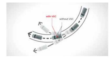
VEHICLE STABILITY CONTROL (VSC) KEEPS YOU IN CONTROL AND THE VEHICLE POINTING STRAIGHT, WHEN ON SLIPPERY SURFACES. IT APPLIES BRAKE PRESSURE TO EACH TYRE INDIVIDUALLY, WHERE NECESSARY.
