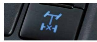
THE REAR DIFFERENTIAL LOCK SYSTEM HELPS SECURE TRACTION WHEN DRIVING IN MUDDY TERRAIN, OR IN THE UNLIKELY SITUATION WHEN THE VEHICLE IS STUCK. THE VEHICLE IS EQUIPPED WITH A SOLENOID SWITCH DIFFERENTIAL LOCK SYSTEM.
