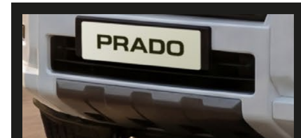
Front Skid Plate To prevent damage during off-roading.
